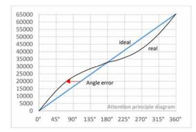
The singleturn repeat accuracy describes the tolerance of the position of the measured and transmitted position value to a reference position or in reverse mode. This means that if the same position or a previously approached reference point is approached several times, the measured and transmitted position value varies with an error in a smaller tolerance band.
