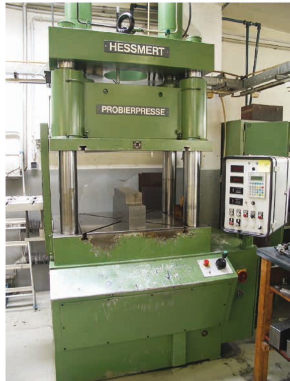
Image 1 The updated tryout press that is used to test the tools
