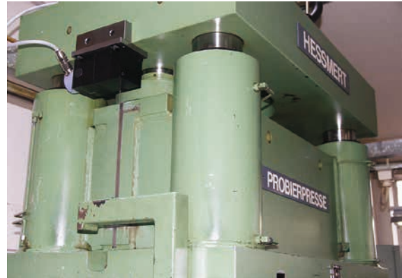
Image 5 Elderly hydraulic press with the latest control technology
