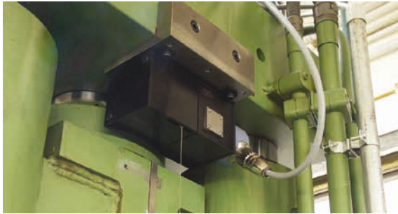
Image 3 The encoder outputs provide signals corresponding to the length of wire paid out, enabling the control software to govern the position of the presses more precisely
