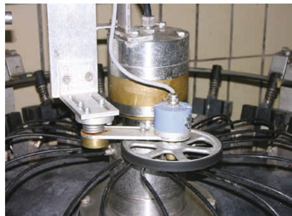
Fig 2: Virtually non-slip application of the measuring device via spring lever and measuring wheel
